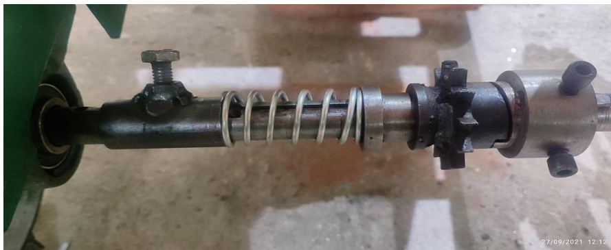
Figure 2. Dog clutch system used for power transmission from ground wheel to metering system
